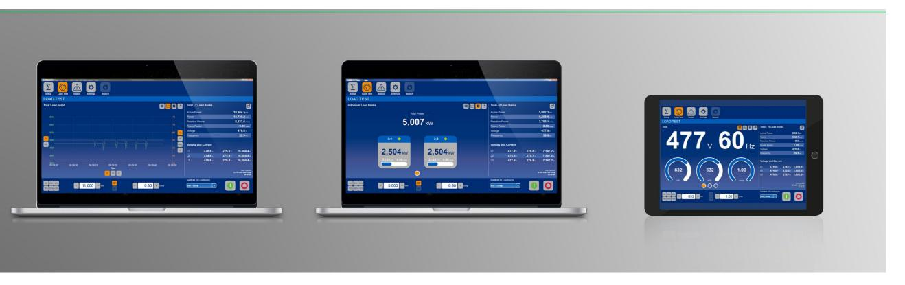
SIGMA PC Basic provides an intuitive user interface with powerful functionality and the ability to control up to 42 load banks in a single network. Load distribution, individual load bank status and control can be accessed when more than one load bank is connected to the network.
