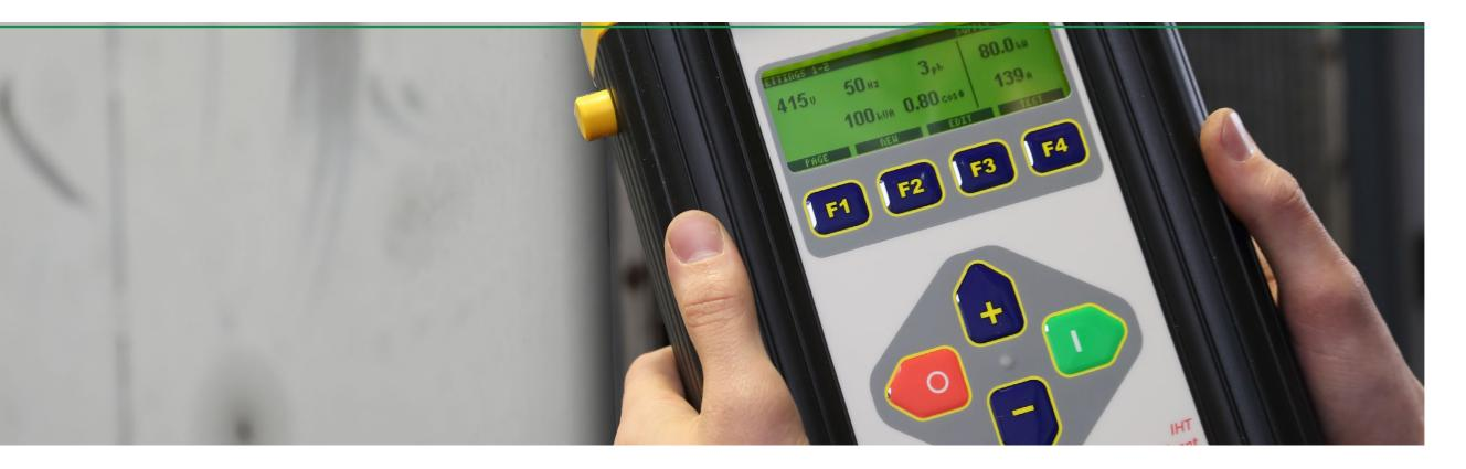
Housed in a robust, industrial polycarbonate enclosure with IP65 protection, membrane keyboard and back-lit graphic LCD, the IHT allows remote load testing with live display information showing all the main electrical parameters. Connect up to 14 load banks in a network with a single IHT for high capacity unity and non-unity power factor testing.
